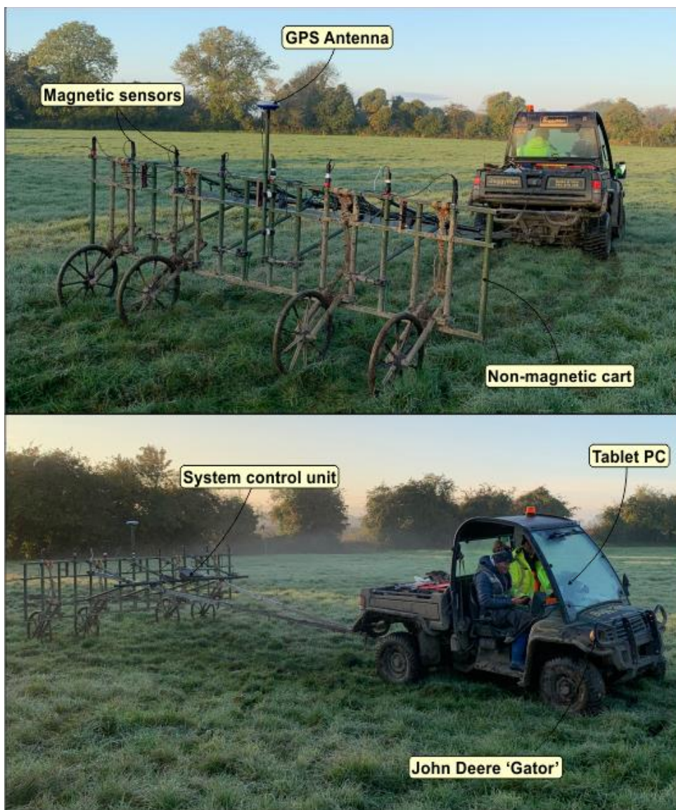
Plate 5: John Deer Gator and Sensys Magneto MXV3 (Library Photo).
